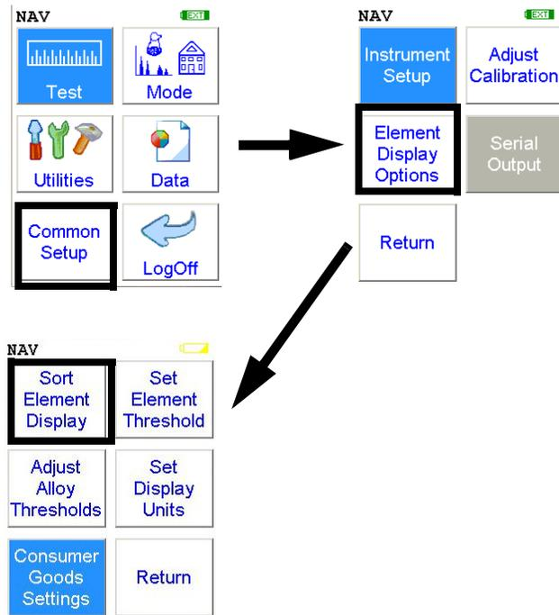
**Figure 1-34. The Sort Element Display Menu Path**
