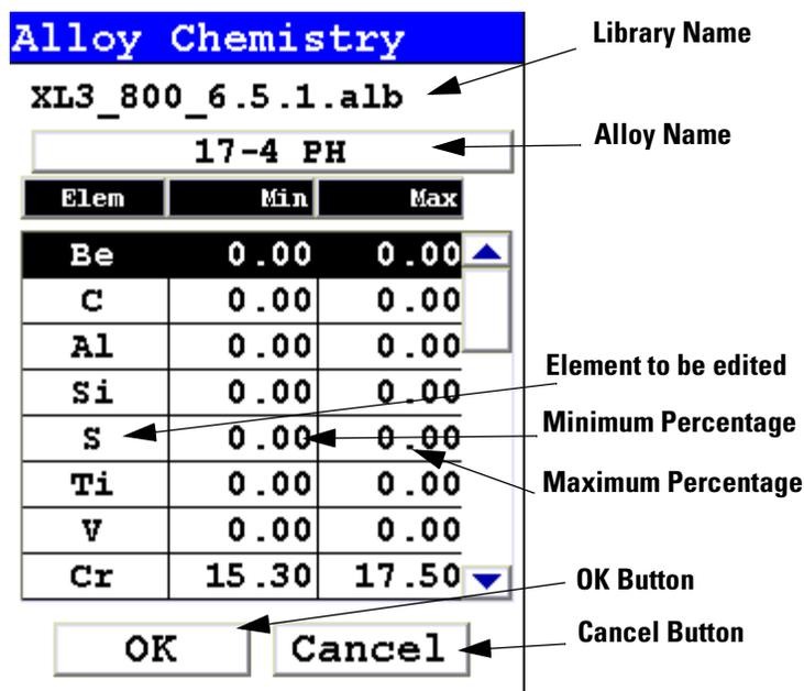
**Figure 1-15. The Element Specification Screen**
