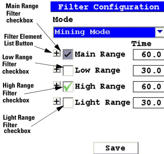
**Figure 1-13. The Filter Checkboxes In Mining Mode**
