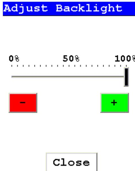
Selecting the red [ - ] box will cause the slider to move some to the left and the screen to dim a bit. Selecting the green [ + ] box will cause the slider to move a bit to the right and the screen to brighten somewhat. Find the setting most harmonious with the ambient lighting. Selecting Close saves the backlight setting in the current state, and returns you to the Utility Menu.
