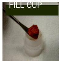
Set the cup on a flat surface film-window-side down. Fill it with at least five grams of the prepared sample, making sure that no voids or uneven layers.
