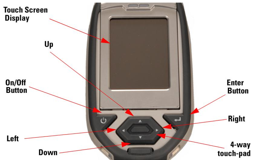
**Figure 1-7. The Control Panel**
