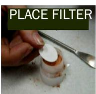
Place a filter-paper disk on the sample after tamping it.
