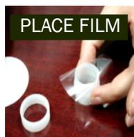
Place a circle of polypropelene film on top of an XRF sample cup. This film goes on the end of the cup with the indented ring. Thermo recommends preparing the cup ahead of time, if possible.
