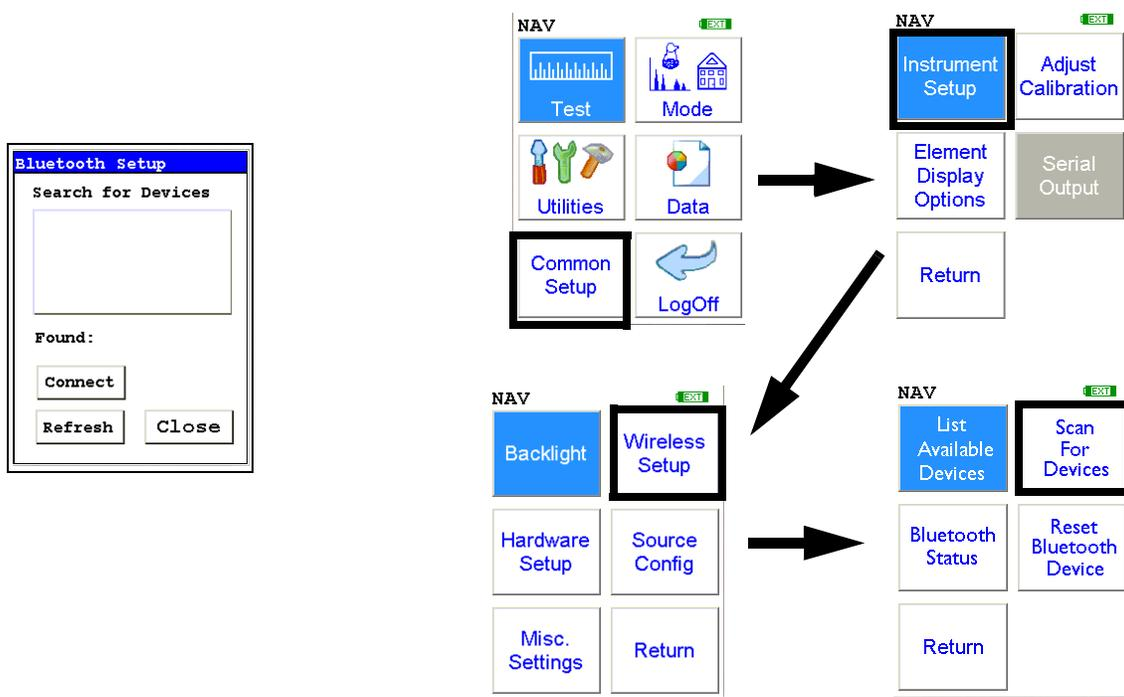
Select the Scan For Devices icon bring up the Bluetooth Search Screen, enabling you to initiate a discovery scan of Bluetooth devices in the operational area. This scan will find all appropriate Bluetooth devices in the operational area, enabling you to connect to those devices.
