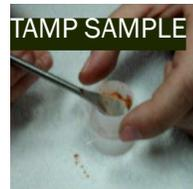
Lightly tamp the sample into the cup. The end of the pestle makes a convenient tamper.
