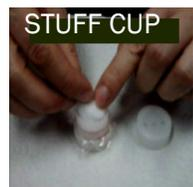
Fill the rest of the cup with polyester fiber stuffing to prevent sample movement. Use aquarium filter or pillow filling as stuffing. A small supply of stuffing comes with your bulk sample kit.
