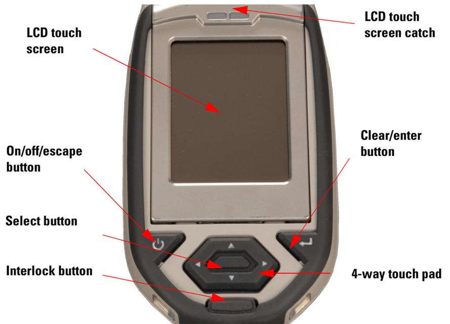
**Figure 0-2. The Control Panel**
