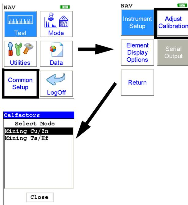
**Figure 1-30. The Adjust Calibration Menu Path**
