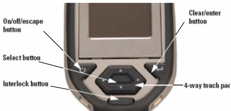
**Figure 1-22. The Control Buttons for the XL3**
