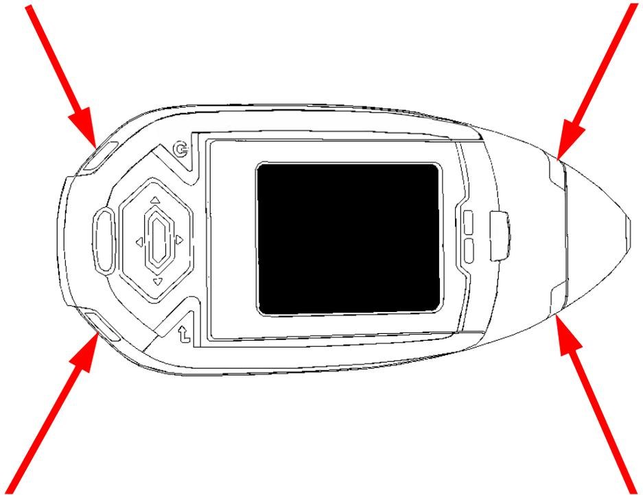
**Figure 3-3. X-ray Beam The Shutter Open Indicator Lights**
