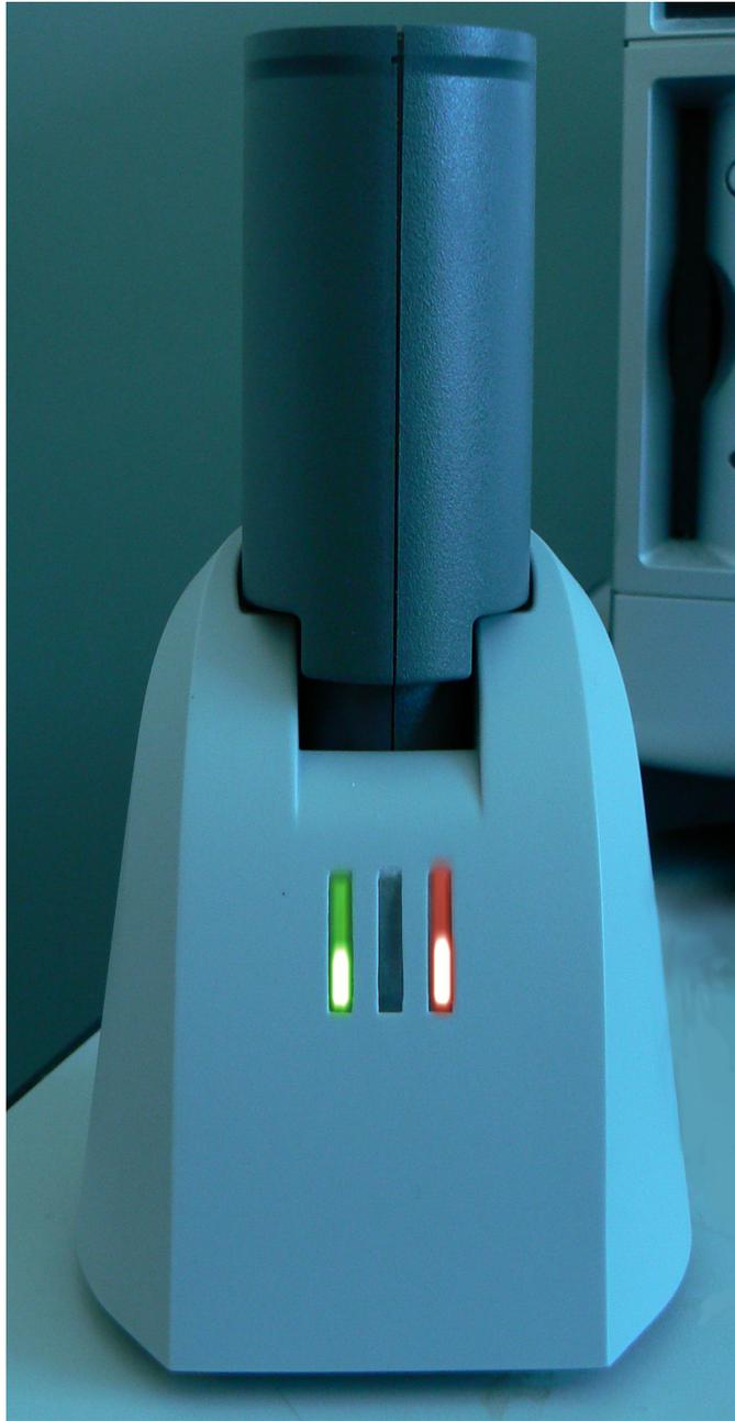
**Figure 2-4. Battery Pack in the Charger**
