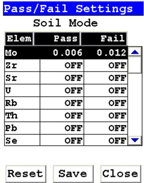
**Figure 1-46. The Settings Screen with new parameters**
