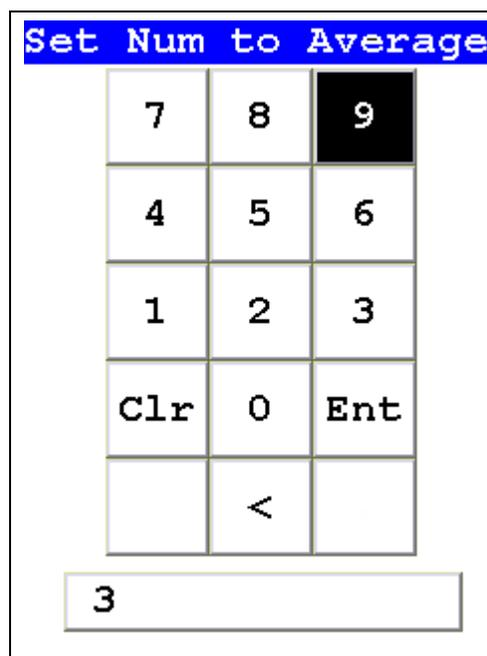
**Figure 1-3. The Virtual Numeric Keypad for Averaging**
