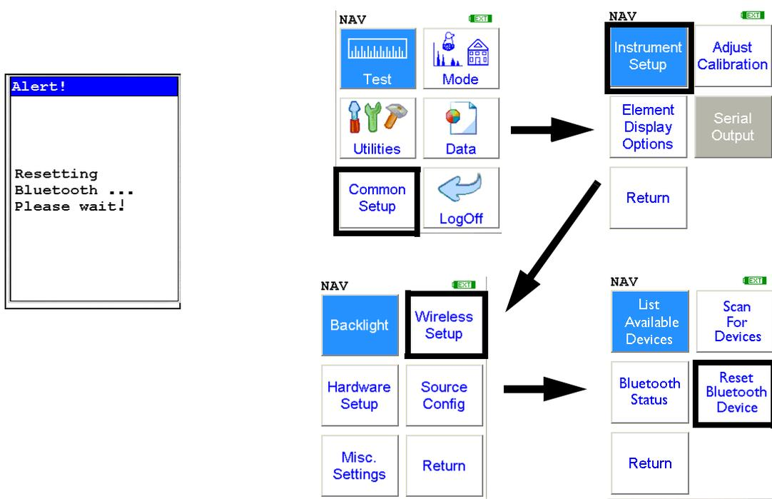
Select the **Reset Bluetooth Device** icon to initiate an immediate reset of the Bluetooth Wireless Networking. Selecting the **Reset Bluetooth Device** icon will clear out old settings and data, as well as enabling you to switch between Bluetooth and standard serial cable. While resetting, your analyzer will show the following screen:
