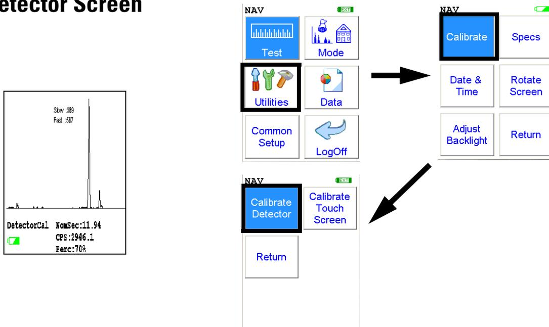
**Figure 1-18. The Calibrate Detector Menu Path**
