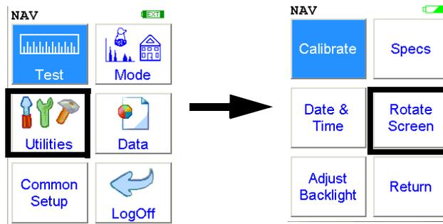
**Figure 1-29. The Rotate Screen 180 Menu Path**
