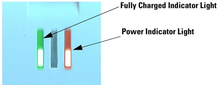
6. If there is a fully seated battery pack in the charger and only the red light is on, there is a fault with the battery pack or charger.
