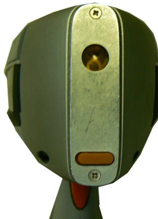
Figure 2-5. View of Face Plate and measurement window
