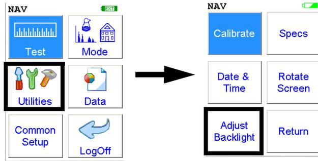
Figure 1-30. The Adjust Backlight Menu Path
