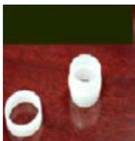
The container used to hold the sample will affect the accuracy of the measurement. Use a container with as thin-walled a window as is convenient and use the same kind of container and window for each sample. Consistency and careful attention to detail are keys to accurate measurement.
